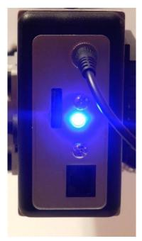
Turn on your smart device and open your networks/Wi-Fi settings. Disconnect from your home network, cellular service, etc. Look for a network connection named "Bullet". Select to connect to it.. The light on the Bullet will turn Blue. Open a browser on your smart device and enter 192.168.4.1 in the URL block at the top. Your browser should now display the main/default screen for the Bullet application. Save the connection to 192.168.4.1 as a bookmark so you can return to it easily in the future.
